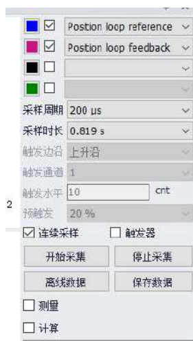
Figure 4-28 Oscilloscope sampling parameters of position loop
