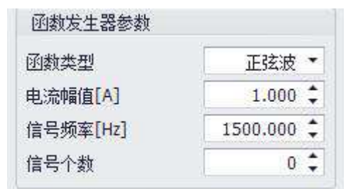
Figure 4-14 Function generator parameters of current loop
