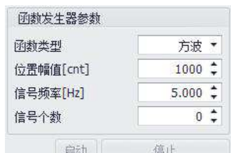
Figure 4-27 Function generator parameters of position loop
