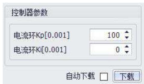
Figure 4-13 Control parameters of current loop
