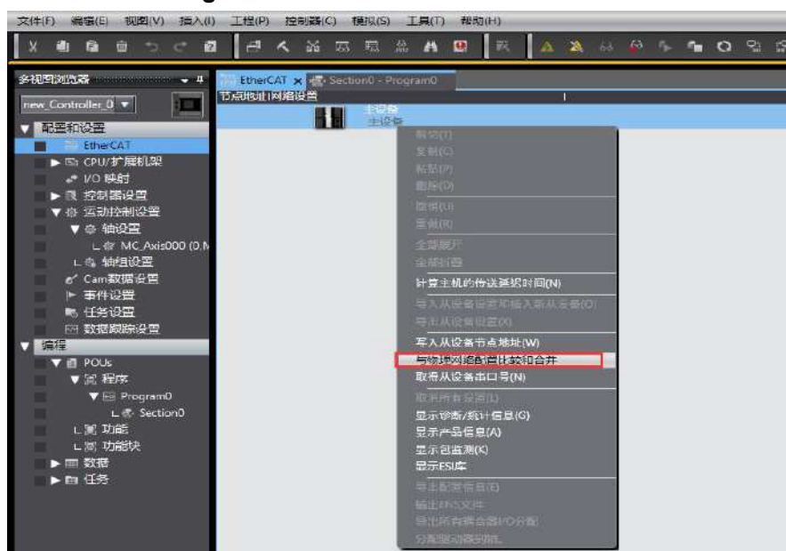
Figure 7-63 Compare and merge interface with physical network configuration
