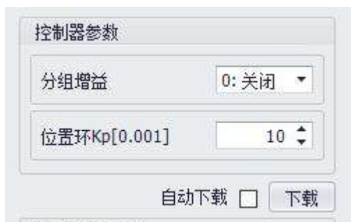
Figure 4-26 Control parameters of position loop
