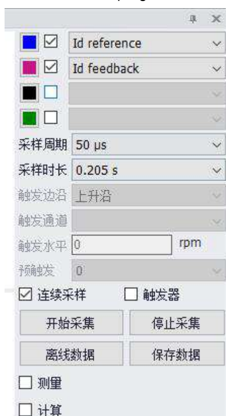
Figure 4-15 Oscilloscope sampling parameters of current loop
