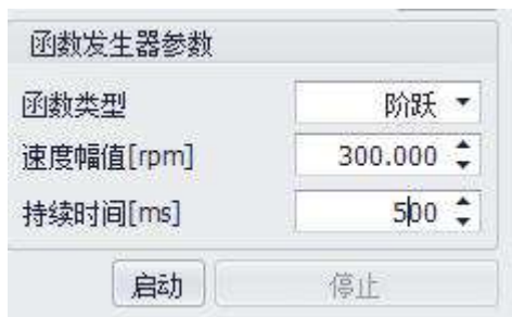
Figure 4-21 Function generator parameters of velocity loop
