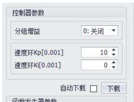
Figure 4-20 Control parameters of velocity loop
