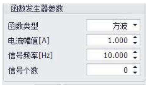
Figure 4-17 Function generator parameters of current loop
