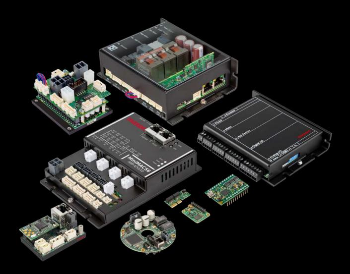
Various 4-quadrant PWM servo controllers for permanent magnetactivated brushed DC motors and brushless EC motors meet all requirements in terms of performance and functionality. Thanks to the fast current controller and dynamic speed controller, outstanding control characteristics are achieved. Combined with maxon high-dynamic motors and Master Controllers, the positioning controllers constitute complete solutions for highly demanding Motion Control applications.
