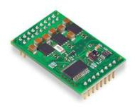
The DEC Module 50/5 (Digital EC Controller) is a 1-quadrant amplifier for controlling EC motors with Hall sensors with a maximum output of 250 watts.
