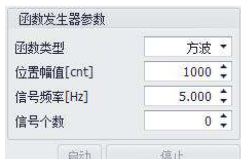
Figure 4-27 Function generator parameters of position loop
