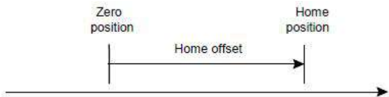
Figure 10-2 Relationship between Zero Point, Origin, and Home Offset
